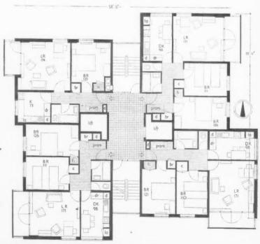
Typical floor plan in point block [Scale: 1/0"]
