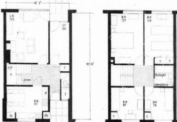
Typical terrace house ground and first floor plans, [Scale:  $\frac{T_0}{T_0}$  = 1'0"]
