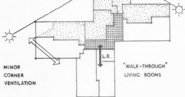
Right, transverse section (Fig. 3) and, below, half-plan (Fig. 4) of typical floor of flats with skip corridor access—an early scheme for Loomis Courts, later abandoned.
