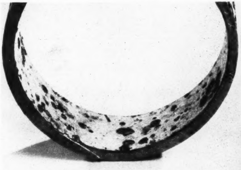
Above, section of steel pipe showing early formation of mushroom heads. Below, left, corrosion mushroom head (slightly less than actual size) removed from internal surface of a water discharge pipe at a large power station; right, reverse side of same mushroom head. Photographs by courtesy of the Factory Painters Ltd., Sheffield.
