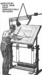
The MAVITTA Drafting Machine stamps your drawing office as EFFICIENT. Made of steel tube with adjustable ball-bearings. The main angles are located automatically, intermediate angles by lock. Scales have inlaid celluloid edges and are divided to order on two edges.
