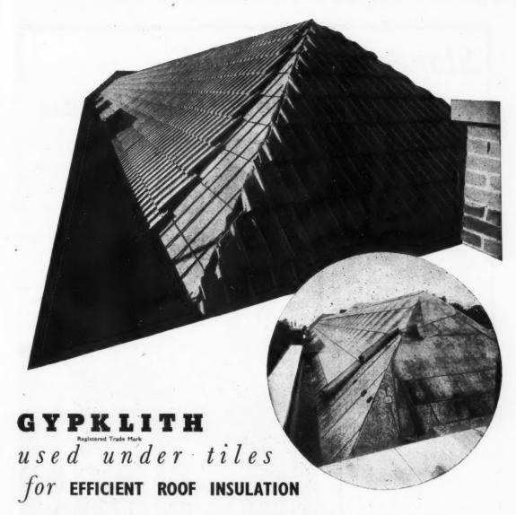
In the roof illustrated, 1½" GYPKLITH is bolted to steel purlins, and covered with bituminous felt. The tiles are secured to "Precision" roofing grillage.
