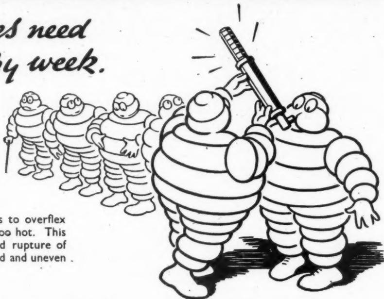
Underinflation causes tyres to overflex when running and to get too hot. This may lead to separation and rupture of the fabric as well as to rapid and uneven wear of the tread.
