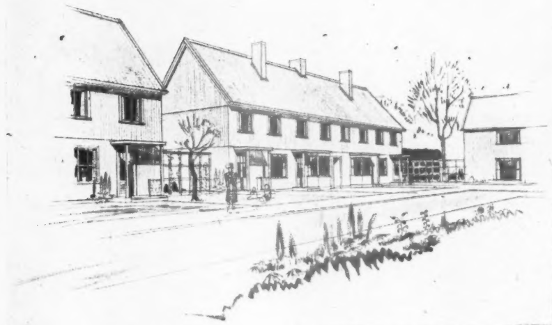
Sketches of two of the designs of Swedish prefabricated permanent timber houses, adapted for Scotland by the Department of Health for Scotland. These are now in production and will soon be arriving in this country. Other plans and designs are now being evolved for England by the Ministry of Works. Top, a pair of the four-roomed, one-and-a-half storey rural type. Below, pairs of the two-storey urban type.
