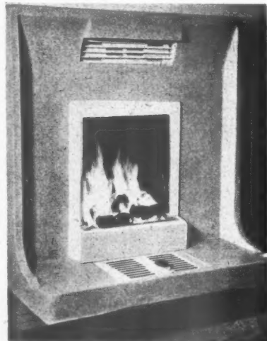
Left, a continuous-burning fire at the Coal Utilization Joint Council's exhibition at the Building Centre. It has air control and underfloor air supply. Warm air is conveyed into the room through the louvres. An ash pit holds a week's ashes. Right, another similar fire showing the closing of the lid used overnight or when the room is not occupied; this obviates the need for relighting. See Astragal's note.
