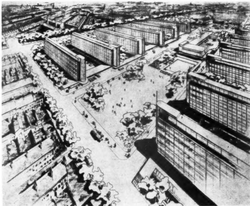
From the film, When We Build Again . The Jewellery Quarter of Birmingham now contains a warren of squalid, cramped and inconvenient factories of the small traditional Birmingham type. Above is an impression of this quarter rebuilt of 5-storey flatted factories, which would contain the same accommodation in the same area as at present. A Welfare Centre is in the middle.
