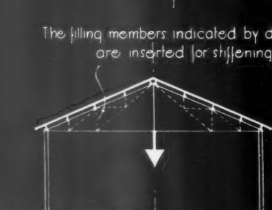
FIGURE 8a: Reasonable shapes of trusses for central loads only
