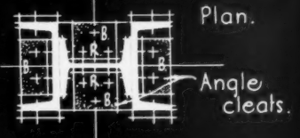
FIGURE 4: SPLICE FOR PARTICULARLY HEAVY COLUMNS.
