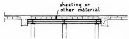
138 Sheetting to be on soffit of slabs, not below beams.
