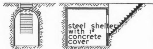
118 Steel shelter, fully sunk in the ground.
