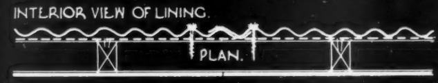
(D) INTERNAL VIEW OF WALL SHOWING THE TYPICAL APPLICATION OF ASBESTOS-CEMENT SHEETING OR ASBESTOS WALLBOARD TO THE INTERIOR.
