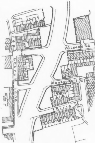
2 Plan of a portion of the New Road as approved by Parliament, showing limits of property which may be bought under compulsory powers.
