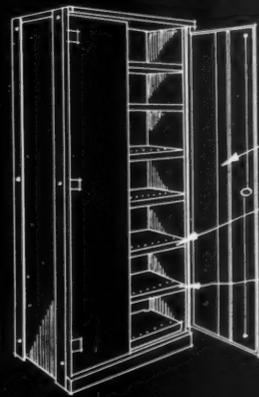
All doors have turned edges and reinforcement down the centre as shown.
