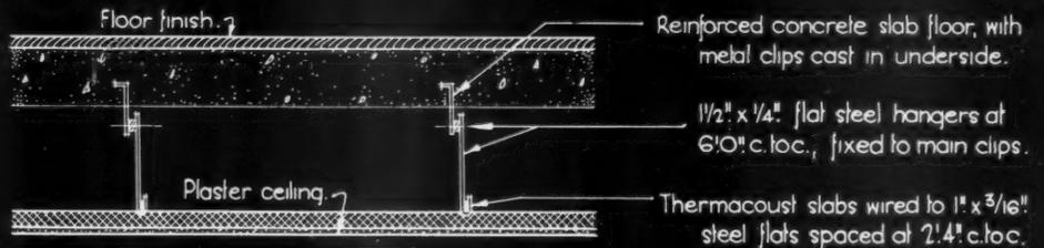
THERMACOUST LAID ON LIGHT STEEL RODS AND RABBIT-WIRED BELOW.
