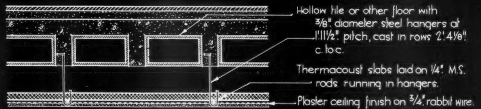
THERMACOUST REBATED OVER CONTINUOUS TEES FOR HEAVY BEARING CONDITIONS.
