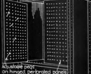
Method of fitting part of a standard shelf unit for storage of tool cutters or gaskets.
