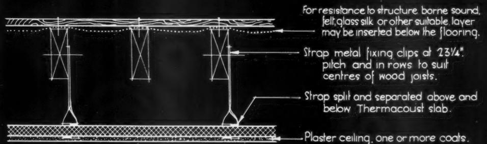
THERMACOUST NAILED DIRECT TO ISOLATED WOOD FLOOR JOISTS.
