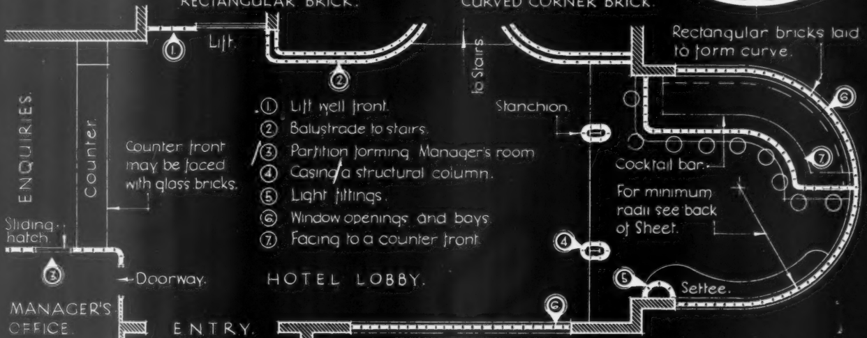
DIAGRAMMATIC PLAN SHOWING SUGGESTED POSITIONS AND TYPICAL USES OF GLASS BRICKS : ILLUSTRATION SHOWS ARRANGEMENT FOR AN HOTEL LOBBY. Scale 1/8" to 1'-0"
