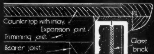
SECTION THRO' COCKTAIL BAR OR COUNTER TOP.
