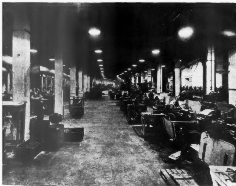
Individual drive : dust hoods over grinding wheels.
