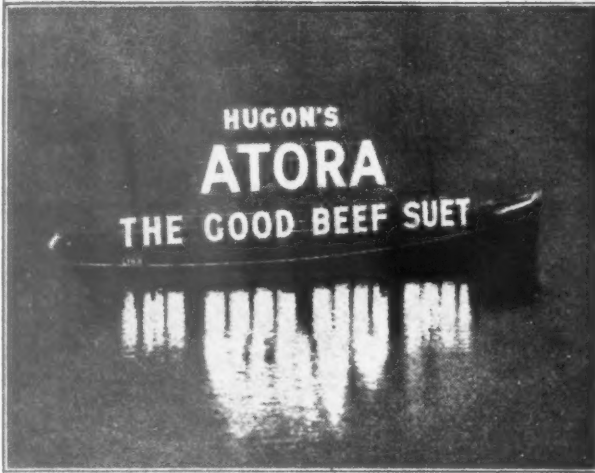
A feature of the Blackpool seascape by night is this ship with the illuminated sign. There have been many conjectures as to the sizes of the letters. Here they are: Hugon's 5ft., Atora 12ft., The Good Beef Suet 7ft. The letters are mounted on tubular steel. The sign is about 100ft. long and 30ft. high, and is worked by special engines and a generator operating three rotary converters.
