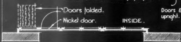
PLAN SHOWING TYPICAL DOOR FIXING (A)
