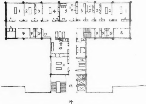
Operating theatre unit at 8th floor level at the Bata Health Centre, Zlín, Czechoslovakia. Architect: Dr. Uklein. An interesting plan showing a twin theatre unit. The provision and position of surgeons' recreation room, blood transfusion room and central sterilizing room should be noted
