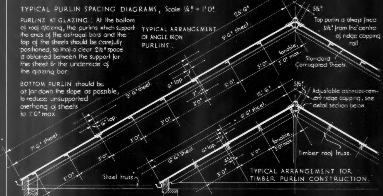
TYPICAL WOOD PURLIN ARRANGEMENT ABOVE & BELOW ROOF GLAZING. Scale : 1/2" equals 1' 0"
