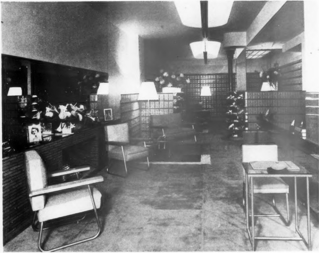
Messrs. Fanchon's shoe shop in Old Bond Street, designed by Mallet-Stevens. The carpet is fawn, chairs are finished in lacquered brass and bright red tapestry, fixtures are natural mahogany and fireplace is in Roman brick and black Vitrolite.
