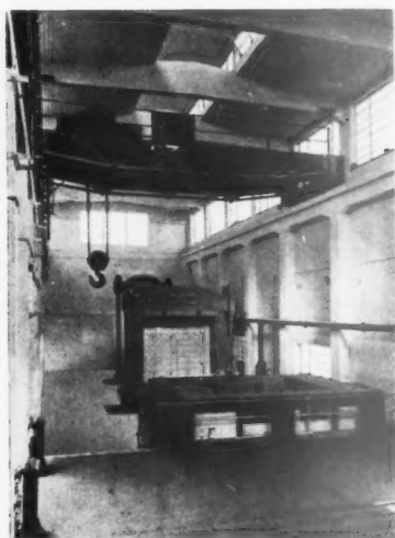
Top: the floor furnace, gas fired; Floor beams to be tested are placed across the top and subjected to heat from below. Below: left, a general view of the test building, with the floor furnace in the foreground and the wall furnace behind it; right, the wall furnace.
