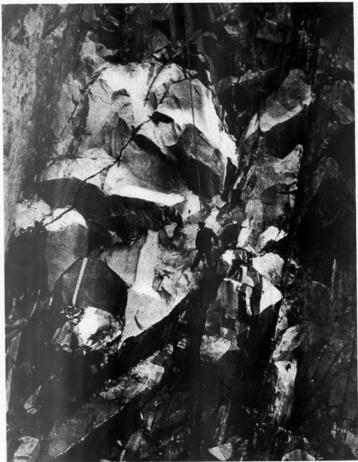
Working out slate rock loosened by blasting; a skilled and often dangerous job.
