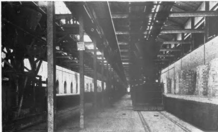
The brick press track at Ridgmont: to the right and left are the kilns, above, the conveyors feeding the ground material to the press hoppers.
