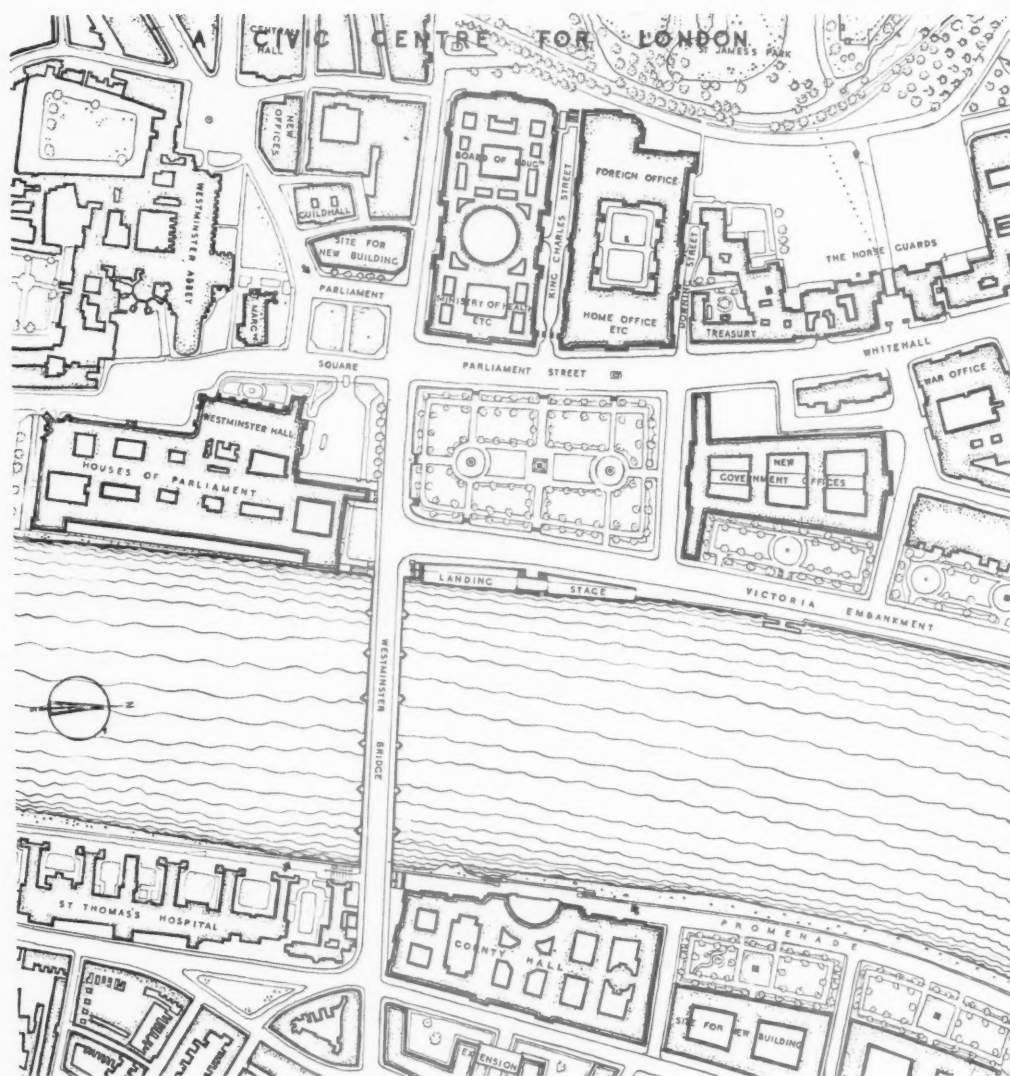
Fig. 3: Plan of the area around the Houses of Parliament, showing the proposed new square, the new Government offices with two side wings added, and new buildings on the west side of Parliament Square and on the east side of the river next to the County Hall. The black arrows indicate the viewpoints of figs. 4, 5, 7 and 8.
