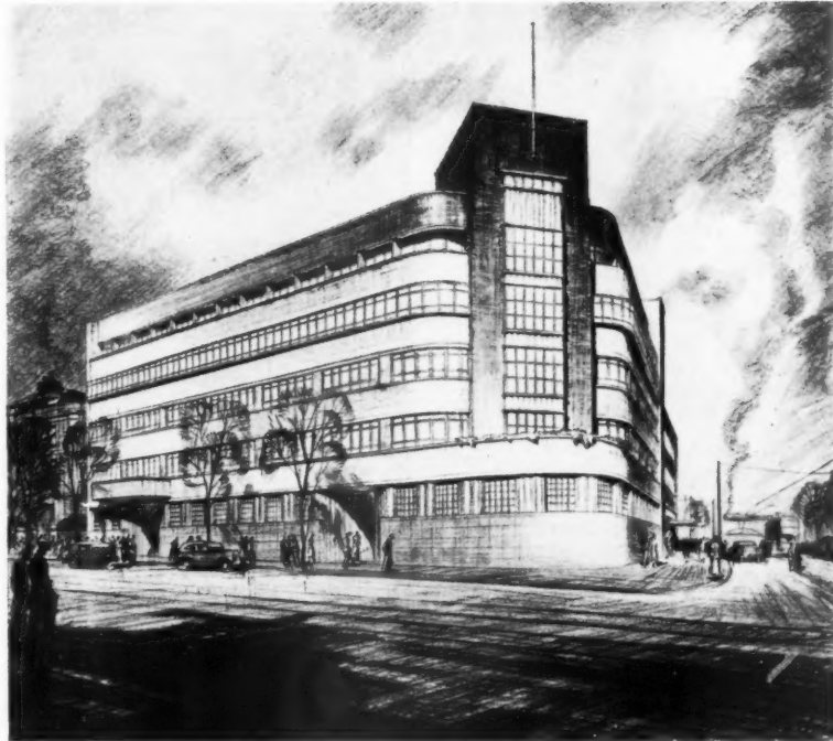
The new Poplar Town Hall on which work was recently begun. The plinth is to be of precast terrazzo, ground-floor piers of green marble, the top banding and tower of thin wide-jointed brickwork, and the remaining wall surfacing of Portland stone veneer. The architects are Messrs. Culpin and Son, and the drawing reproduced is by Mr. J. D. M. Harvey.
