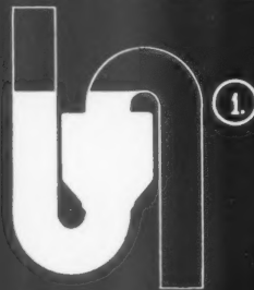
1. The trap under normal conditions giving a seal of 4\frac{3}{4} ".
