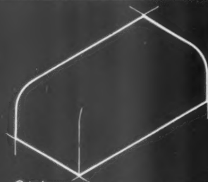
BULLNOSE INTERNAL RETURN ON FLAT.
