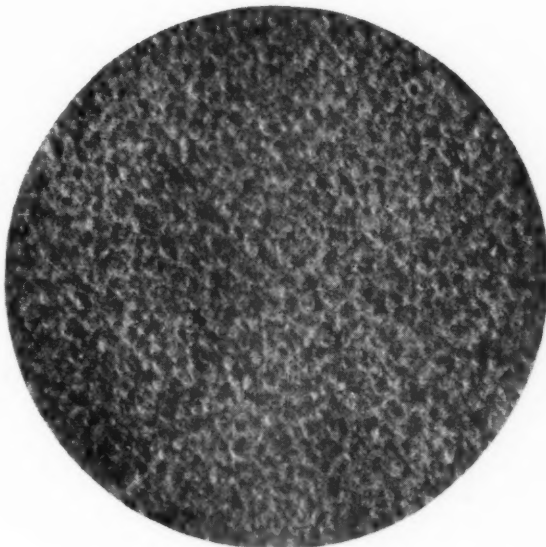
Above, a mixture of wood flour and fine sand sprayed upon a "tacky" undercoat over which a finishing coat of some desired colour has been applied. Below, finely-ground cork dust applied to a "tacky" undercoat with thick coats of flat paint to give the finished surface.
