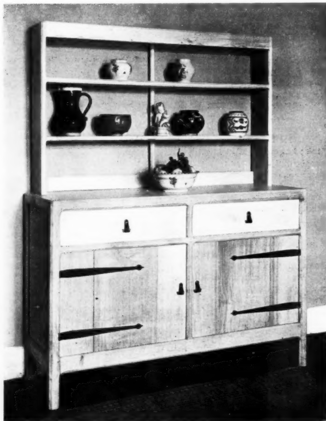
An early example of a simple dresser in oak. Severely plain, it is a straightforward and workmanlike job. The drawer handles are obviously too small, but in the matter of handles there is much more to say. Craftsman, G. Cook.
