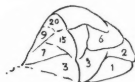
FIG 6 HOW HOT LIME GETS INTO THE WALL & CAUSES IT TO LIFT & CRACK. ADDITIONS OF NEWLY MIXED MORTAR SHOULD NOT BE PLACED SO THAT THEY WILL BE USED FIRST - 20 BEFORE 1 ETC.
