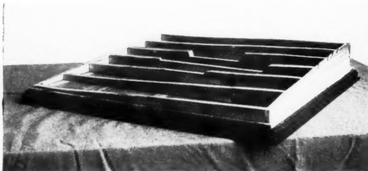
FIGURE SIX.—BASEBOARD WITH CONTOUR STRIPS IN PLACE.
