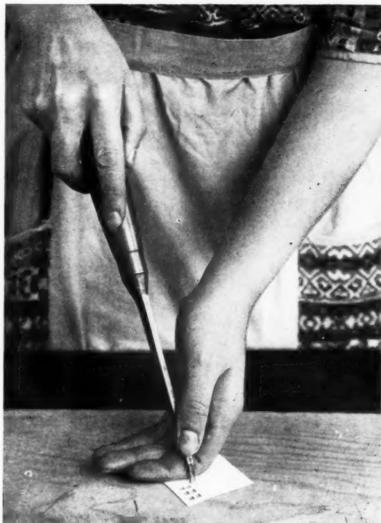
FIGURE FOUR.—CHISEL FOR CUTTING SMALL APERTURES.
