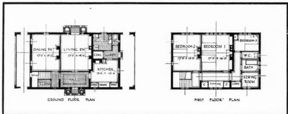
GROUND- AND FIRST-FLOOR PLANS
