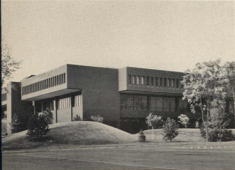
Systems Development Laboratory, International Business Machine Corporation, Poughkeepsie, New York, has cantilevered top floor and punched fenestration to break up monolithic appearance of the 464x224-foot structure. Principals in charge: Willis N. Mills Sr., FAIA; A Raymond von Brock, AIA; designer: Willis N. Mills Jr., AIA.
