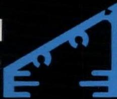
NEW Amarlite Vault Action Windows feature a bank-vault style smooth sloped sill and frame . . . creates a self-wedging seal that defies the weather. New sill design eliminates weep holes . . . water dams . . . and minimizes dust and dirt accumulation. Heavy duty, adjustable friction hinge holds window firmly open . . . glass easily replaced from the inside. Fast delivery to the job site on a complete variety of standard sizes. See Sweet's, our representative, or write us.
