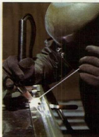
Door stiles, top and bottom rails are accurately fitted and continuously welded. All joints are flush . . . no projections or offsets.
