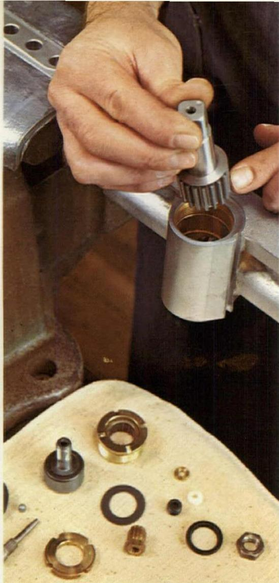
All components are pre-fitted and tested at the factory. Each hydraulic cylinder, for example, is given an operational, break-in test before actual installation in the door.
