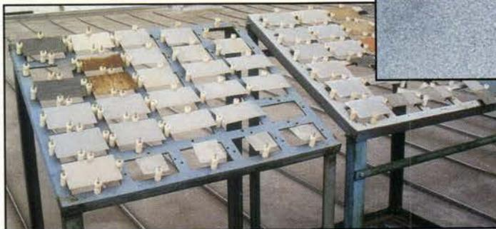
In addition to extensive laboratory testing at California State University at Berkeley, Follansbee exposed samples to salt-laden beach front exposure for more than 5 years at a test site in Topsail, North Carolina.
