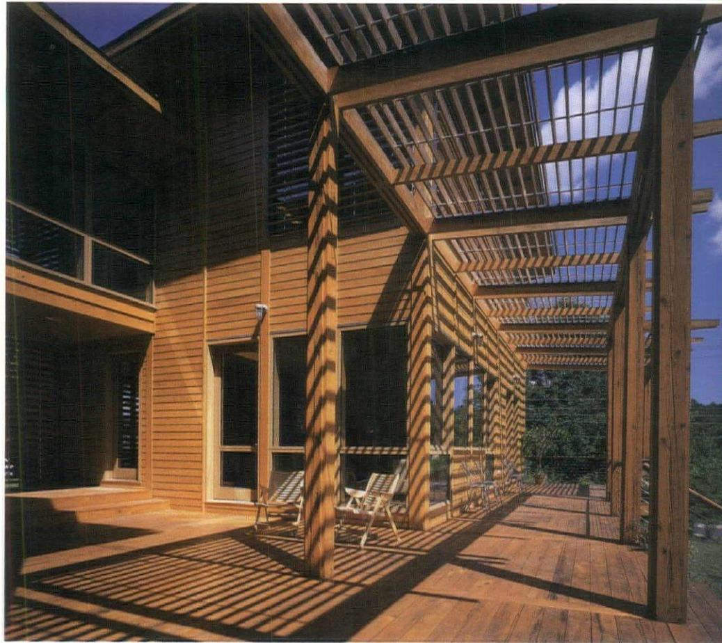
Louvers that shade the upper-floor windows turn horizontally and become latticework on the trellis (above). The two sections of the house frame a view of the landscape (below).
