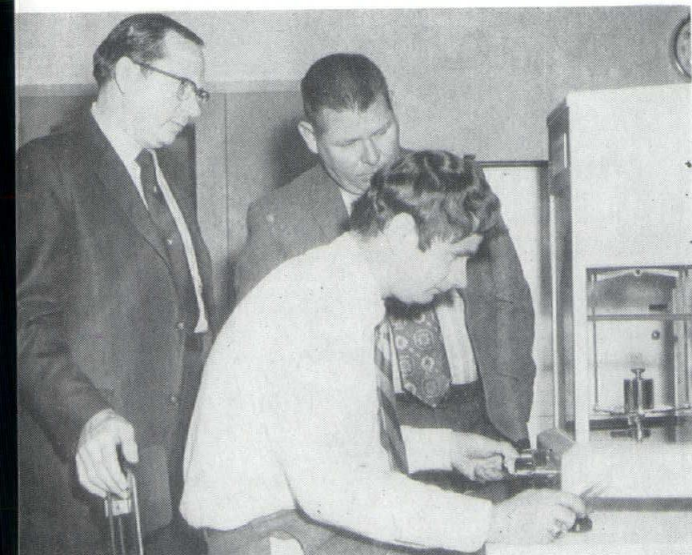
James F. Lyles (right) supervisor of the weights and measures section, and James C. Stewart, assistant supervisor, watch as Marion W. Cain, state metrologist calibrates a precision 5 pound mass standard.
