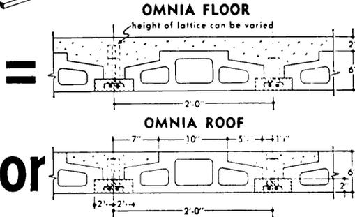
The OMNIA floor is monolithic in character and behaves structurally like a floor slab cast in place, yet requires no forming. It is lightweight and economical.
