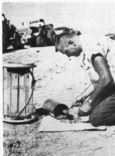
Checking compacted fill for density determination with water-balloon method, a typical step in testing and control by Engineers Testing Laboratories, Inc.
