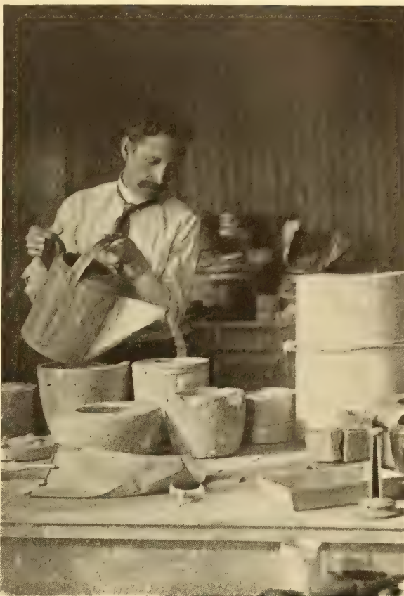
Pouring the slip into the mold
