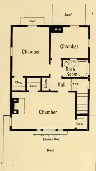
Fig. 30—Second floor plan
