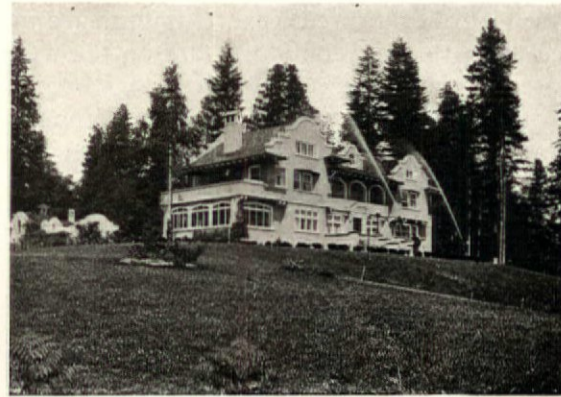
Two streams may be thrown over the house, using 1 1/2 inch hose and 1/2 inch nozzles
