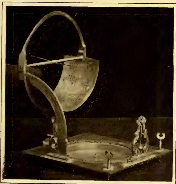
A Brass Sun-dial with Plumbob for Leveling
