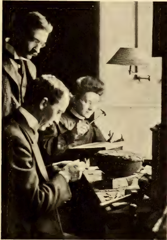
Students at Work. The Girl with the Hammer is Working on a Sheet of Brass Screwed on a Flat Piece of Wood
