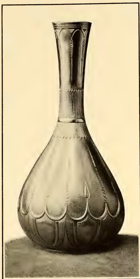
In Making this Type of Ware Specially Contrived Gauges Are Fitted Into the Object and the Design Worked-up on the External Face
