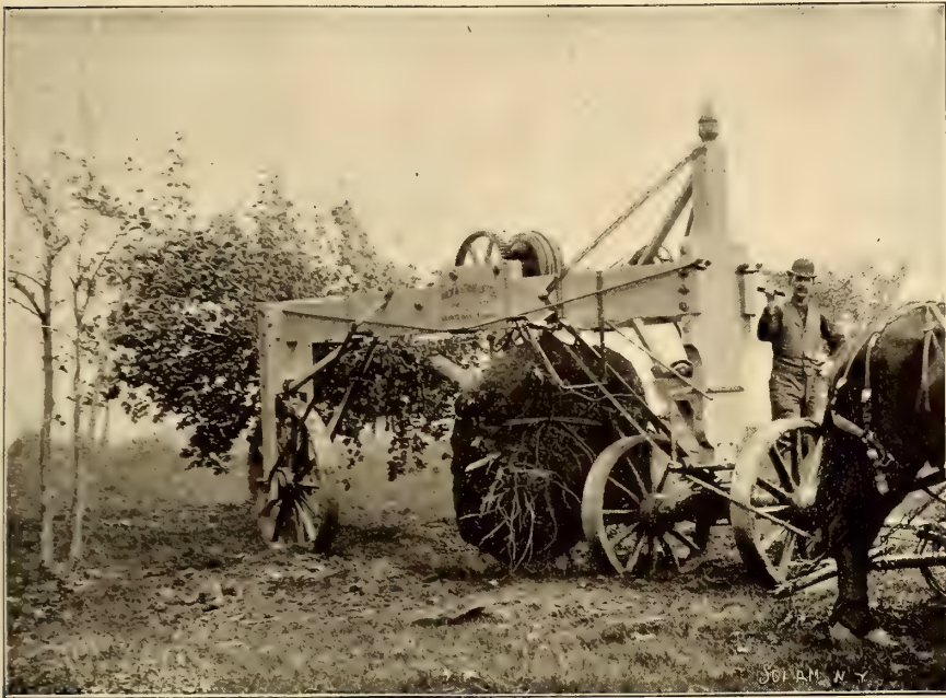
A Powerful Machine for Moving Rocks and Large Trees
