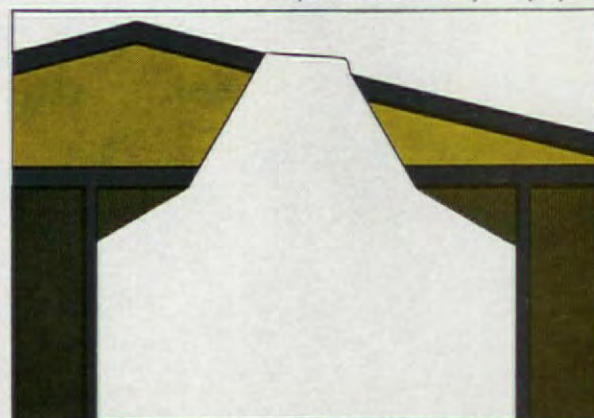
For better spread of light for larger rooms, sides of shaft may be splayed.
