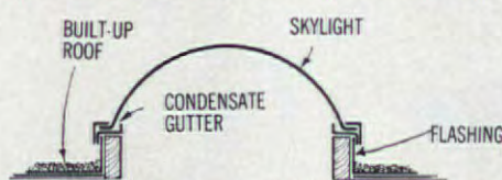
An important part of many skylights is the gutter, which catches moisture condensing on dome.
