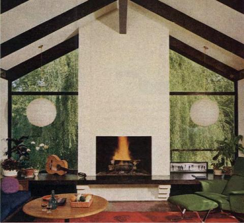
Fireplace in a remodeled home in Connecticut is stucco over concrete block. The hearth ledge extends across the room and is made of painted, reinforced concrete. Picture windows look to the deck and yard. Dark beams provide contrast for the white walls.
