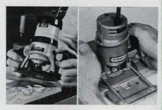
guide for straight and circular cuts. Manufacturer is The Stanley Works, New Britain, Conn. The other is a Green Line ½-hp, 28,000-rpm unit from Rockwell Manufacturing of Pittsburgh, Pa. It sells for \$39.95. Both tools take bits with ¼-inch shanks. Both these tools are more than adequate for the home shop.
