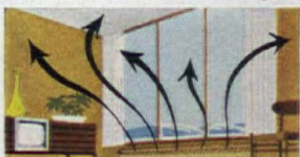
Baseboard units save space, permit room-by-room temperature control. Radiant or hot water types available.
