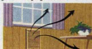
Wall panel, with heating units behind grille, provides radiant heat with natural or fan-forced convection.
