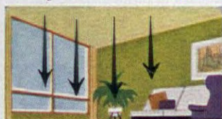
Radiant ceiling heat: concealed within ceiling. Each room's temperature can be individually controlled.
