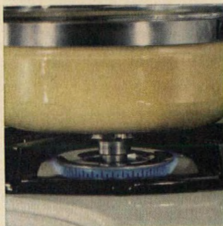
Burner operates on full flame (left) until the food reaches selected temperature, then lowers automatically (right) until the sensing element calls for more heat—much like an oven thermostat. Foods won't scorch when heat is measured as accurately as any other ingredient you use. Electric ranges are available with similar surface cooking controls, some of which provide for adjustment according to size of pan.
