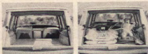
Back end stays level. Optional air units automatically level wagon when you're carrying heavy loads or hauling a trailer.
